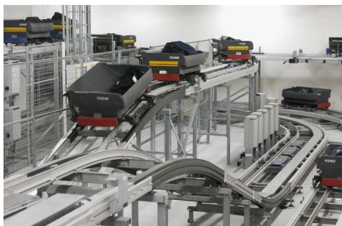
Fig. 16.1 DCVs running on a network of tracks (Photo courtesy of Vanderlande Industries)
