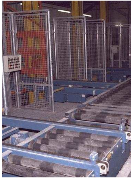
Fig. 17.1 Pallet elevators at the distribution center of Herlitz with a single waiting slot in front of each
