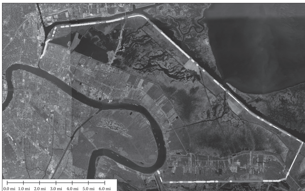
Figure 23.20 Pre-Katrina crown deviation from design elevation relative to mean sea level for the Chalmette levee loop (white = at design el., all other up to 3.0 feet too low). (From Shaffer, G.P. et al., J. Coastal Res. , 54, 206–224, 2009; Morris, 2008.)
