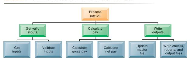
This structure chart shows the highest or most abstract level of design for a payroll system, providing an overview of the entire system.
