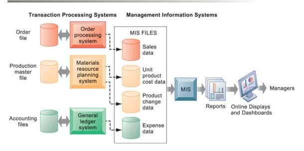
In the system illustrated by this diagram, three TPS supply summarized transaction data to the MIS reporting system at the end of the time period. Managers gain access to the organizational data through the MIS, which provides them with the appropriate reports.
