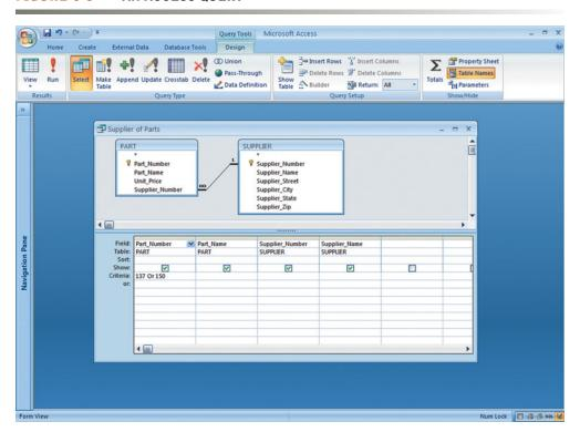
Illustrated here is how the query in Figure 6-7 would be constructed using Microsoft Access query-building tools. It shows the tables, fields, and selection criteria used for the query.
