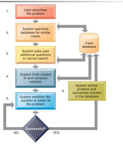
Case-based reasoning represents knowledge as a database of past cases and their solutions. The system uses a six-step process to generate solutions to new problems encountered by the user.
