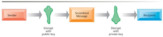
A public key encryption system can be viewed as a series of public and private keys that lock data when they are transmitted and unlock the data when they are received. The sender locates the recipient's public key in a directory and uses it to encrypt a message. The message is sent in encrypted form over the Internet or a private network. When the encrypted message arrives, the recipient uses his or her private key to decrypt the data and read the message.
