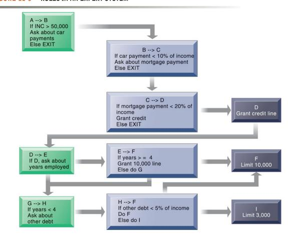
An expert system contains a number of rules to be followed. The rules are interconnected; the number of outcomes is known in advance and is limited; there are multiple paths to the same outcome; and the system can consider multiple rules at a single time. The rules illustrated are for simple credit-granting expert systems.
