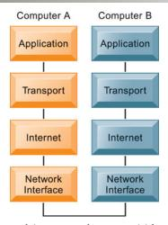
This figure illustrates the four layers of the TCP/IP reference model for communications
