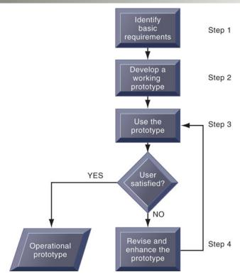
The process of developing a prototype can be broken down into four steps. Because a prototype can be developed quickly and inexpensively, systems builders can go through several iterations, repeating steps 3 and 4, to refine and enhance the prototype before arriving at the final operational one.
