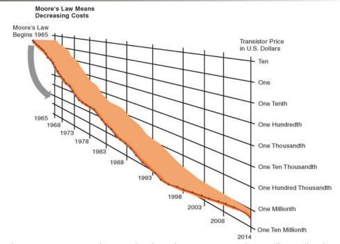
Packing more transistors into less space has driven down transistor cost dramatically as well as the cost of the products in which they are used.
