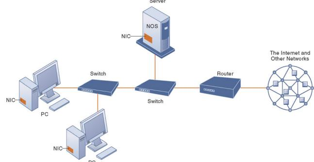
Illustrated here is a very simple computer network, consisting of computers, a network operating system residing on a dedicated server computer, cable (wiring) connecting the devices, network interface cards (NICs), switches, and a router.
