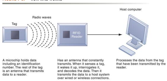
RFID uses low-powered radio transmitters to read data stored in a tag at distances ranging from 1 inch to 100 feet. The reader captures the data from the tag and sends them over a network to a host computer for processing.
