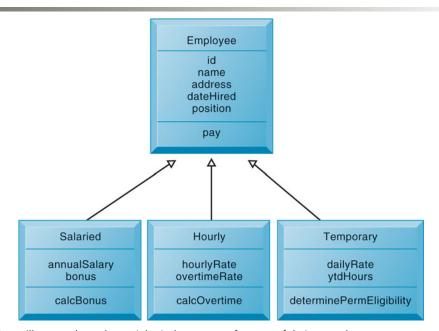
This figure illustrates how classes inherit the common features of their superclass.
