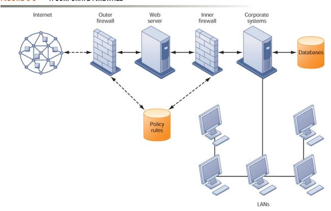
The firewall is placed between the firm's private network and the public Internet or another distrusted network to protect against unauthorized traffic.
