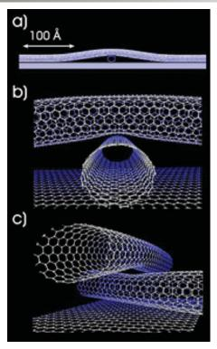
Nanotubes are tiny tubes about 10,000 times thinner than a human hair. They consist of rolled up sheets of carbon hexagons and have the potential uses as minuscule wires or in ultrasmall electronic devices and are very powerful conductors of electrical current.
