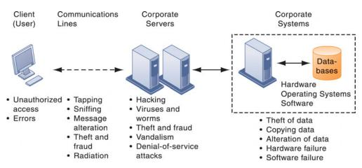
The architecture of a Web-based application typically includes a Web client, a server, and corporate information systems linked to databases. Each of these components presents security challenges and vulnerabilities. Floods, fires, power failures, and other electrical problems can cause disruptions at any point in the network.
