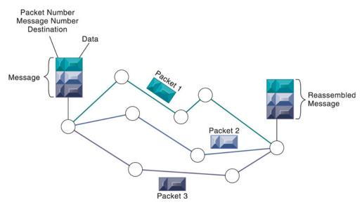
Data are grouped into small packets, which are transmitted independently over various communications channels and reassembled at their final destination.
