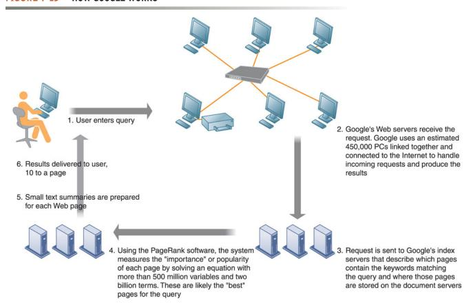
The Google search engine is continuously crawling the Web, indexing the content of each page, calculating its popularity, and storing the pages so that it can respond quickly to user requests to see a page. The entire process takes about one-half second.
