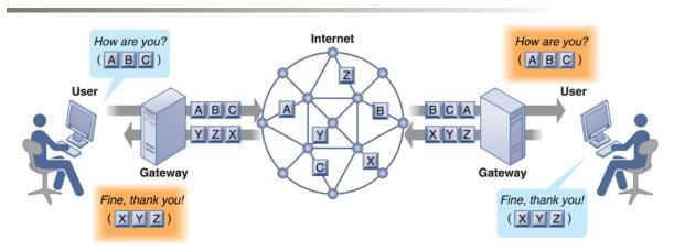
An VoIP phone call digitizes and breaks up a voice message into data packets that may travel along different routes before being reassembled at the final destination. A processor nearest the call's destination, called a gateway, arranges the packets in the proper order and directs them to the telephone number of the receiver or the IP address of the receiving computer.
