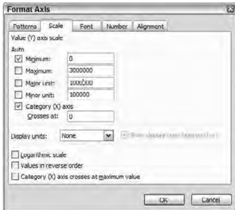
Figure 19.10: Clear the check boxes and use large Major Unit values on the Scale tab to remove unnecessary numbers along the Y-axis.
