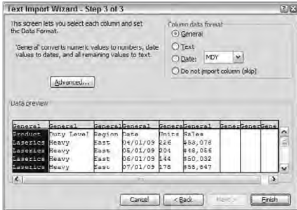
Figure 28.4: Step 3 of 3 in the Text Import Wizard enables you to set column formats if Excel does not choose correctly.
